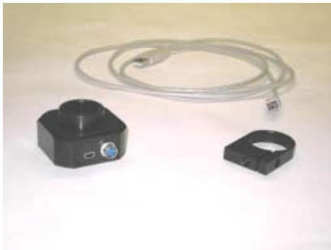
1B. Screw your half-inch camera lens onto the front of the camera.
