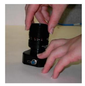
1B. Screw your half-inch camera lens onto the front of the camera.
