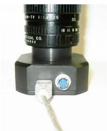
1D. Connect the camera to the USB 2.0 port on your computer with the USB cable.
