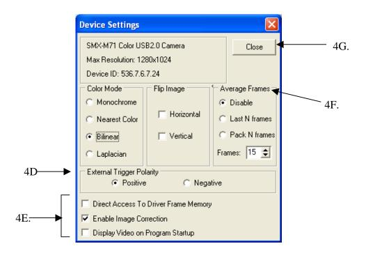
4D. **External Trigger Polarity**: This option is for taking snapshots with an external trigger. "Positive" enables the Trigger input #1, and Negative enables trigger input #2. For more information, see the External Trigger Connector diagram in the User Guide.
